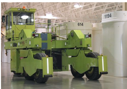
Used fuel in an on-site transport vehicle
