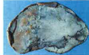
Found in clay-rich mudstone, this 12-centimetre copper plate experienced little-to-no corrosion for 200 million years.
